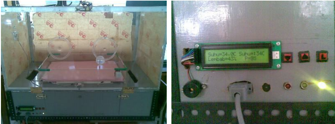
Gambar 7. Realisasi purwarupa inkubator digital
