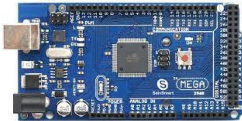
Gambar 3. Arduino mega 2560
