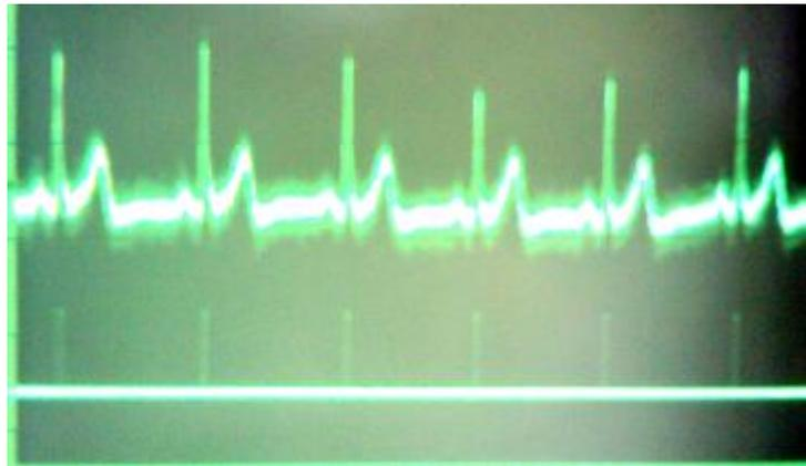
Fig. 17. Detected R points of a ECG signal
